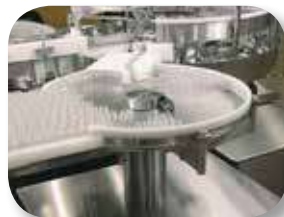
Downed vial reject systems
